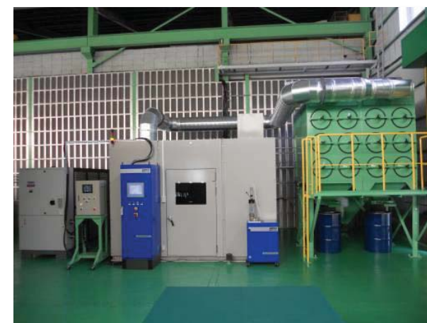
HVOF Coating Equipment No.1 (φ200×L800 mm Max.30 kg)
