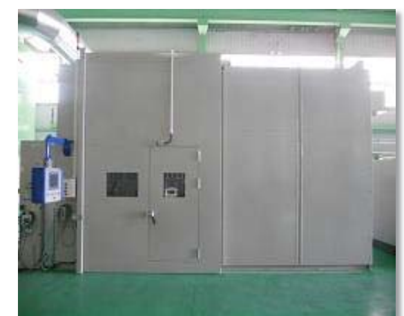
HVOF Coating Equipment No.2 (φ400×L2,000 mm Max.150 kg)
