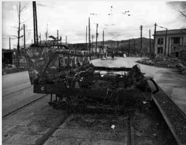
A-bombed 100 Series (Car 115) streetcar near the Yokogawa Line terminal. It was a wooden streetcar that began operation in 1912, so only the burned platform remained. (Courtesy of Hiroshima Peace Memorial Museum, Photo by the US military)
