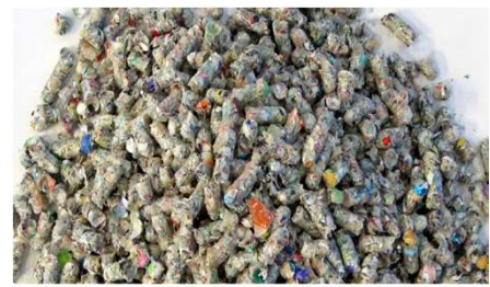
RDF production plant: Solid fuel production from municipal solid waste and/or industrial waste. ¥
