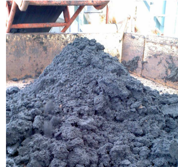
Dewatered cake from a decanter
