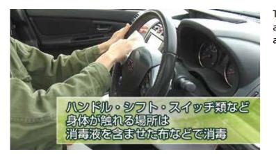
To disinfect interior parts touched by hand, such as the steering wheel, gear shift and switches, use a cloth moistened with disinfectant.
